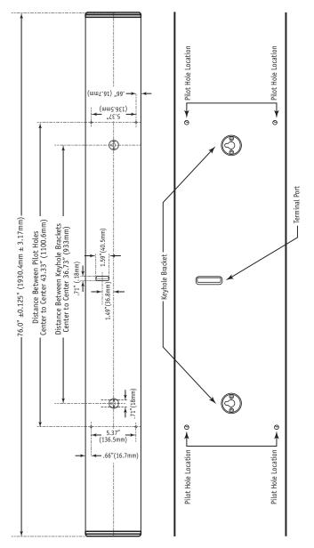
Back diagram for the Ultra-3 soundbar showing the keyhole brackets, pilot holes and terminal port.
