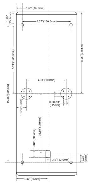
Back diagram for the Ultra-1 on-wall speaker showing the keyhole brackets, pilot holes and terminal port.
