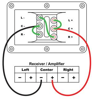
How to wire all channels of the Ultra-3 for use as a single channel.
