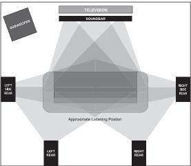
thinner than if the woofer were close to a wall. Good results can usually be obtained by placing a subwoofer along a wall 1-3 feet from a corner. Experiment with subwoofer placement and the sub-amplifier controls to achieve the proper bass balance.
