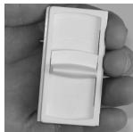
5.) Once the new slide knob is in the new faceplate, check to make sure it slides easily in the slot.
