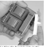
7.) Align the faceplate tabs in the top two holes in the metal back plate. Then, make sure the other two plastic tabs align with the other two holes in the metal back plate.
